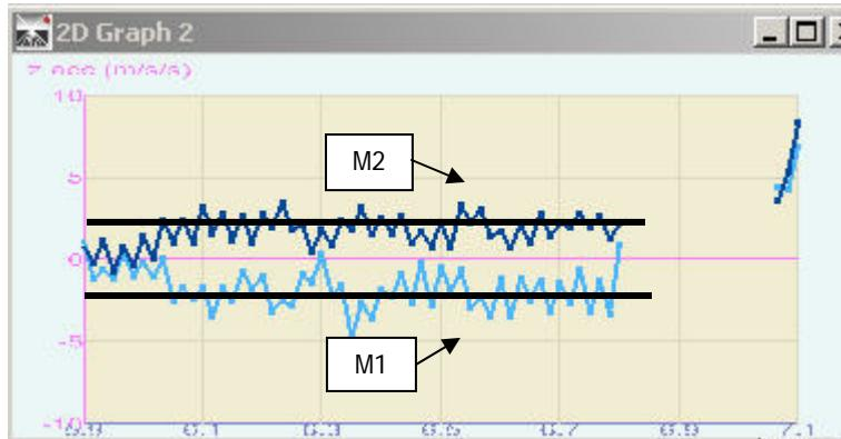
When the 200 gram hanging mass is released, it supplies the force that accelerates the 100 gram hanging mass. If friction effects and the masses of the string and pulley are ignored, then the approximate average acceleration of the system is given by the above graph.
