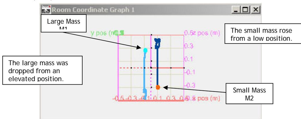
2. **Z Position v. Time Graphs:** Graphical interpretation of the masses' displacement in the Z-direction.
