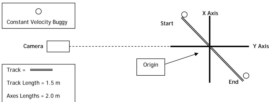
In this activity, the buggy moved from quadrant III to quadrant I of the Cartesian coordinate system, passing very close to the origin. This motion shows up when viewed in the Room Coordinate Graph. Any path could be taken and we encourage you to try different various directions to compare and contrast the data.
