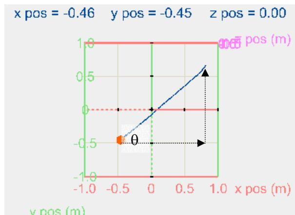
The correlation between this graph and the separate X Position v. Time and Y Position v. Time graphs can be shown by calculating the same angle this time by finding the displacement in both planes on the X and Y Position v. Time graphs.
