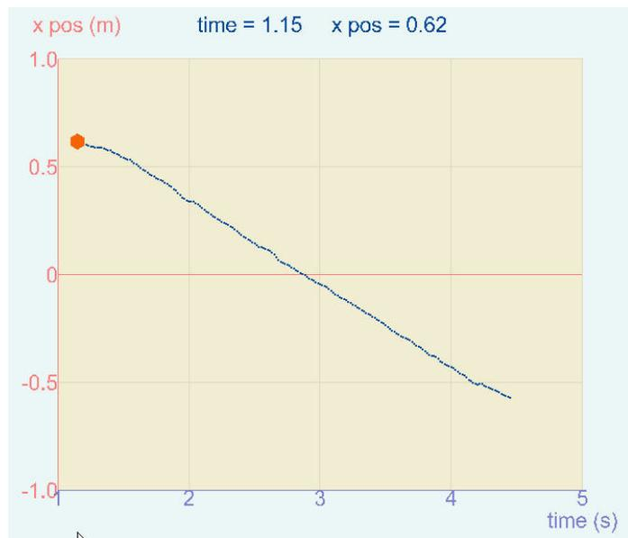
The average velocity can be determined quantitatively by calculating the slope of this line.
